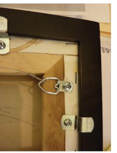
Example of properly installed D ring
